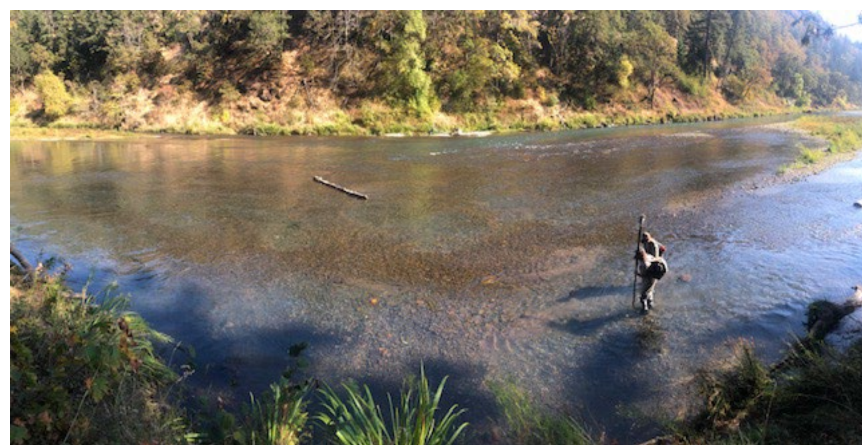
Figure 2. Ground surveyors mapping redds with ArcGIS Field Maps and an Arrow RTK GNSS Receiver (cm level accuracy).
