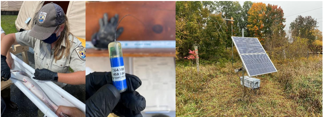
Figure 2. Radio tagging Atlantic salmon (left image), Sigma Eight Inc. radio telemetry transmitter (center image), and Sigma Eight Inc. radio telemetry receiver in the Winooski River.
