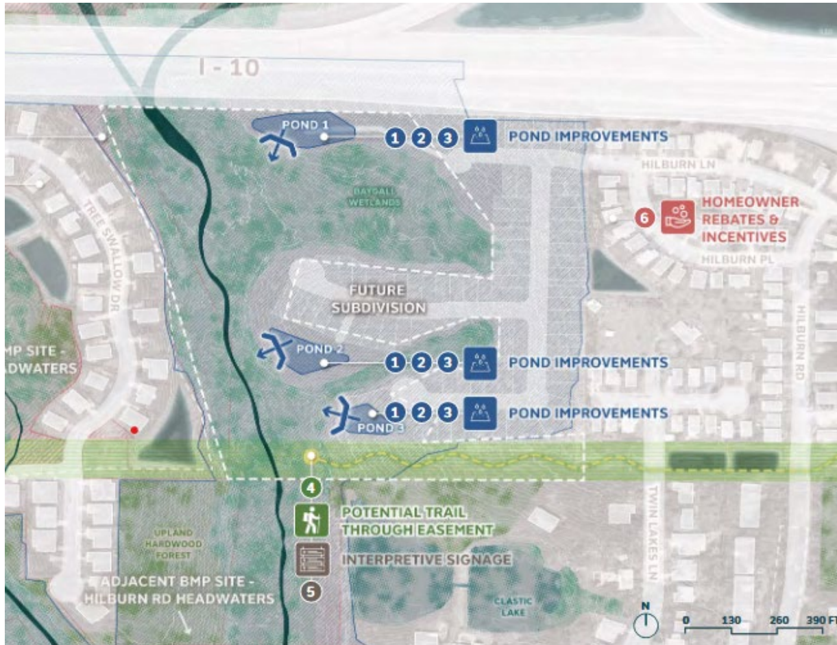
Figure A-4 Conceptual Drawing of the Installations at the Existing Stormwater Pond South of I-10 (Escambia County, 2022)
