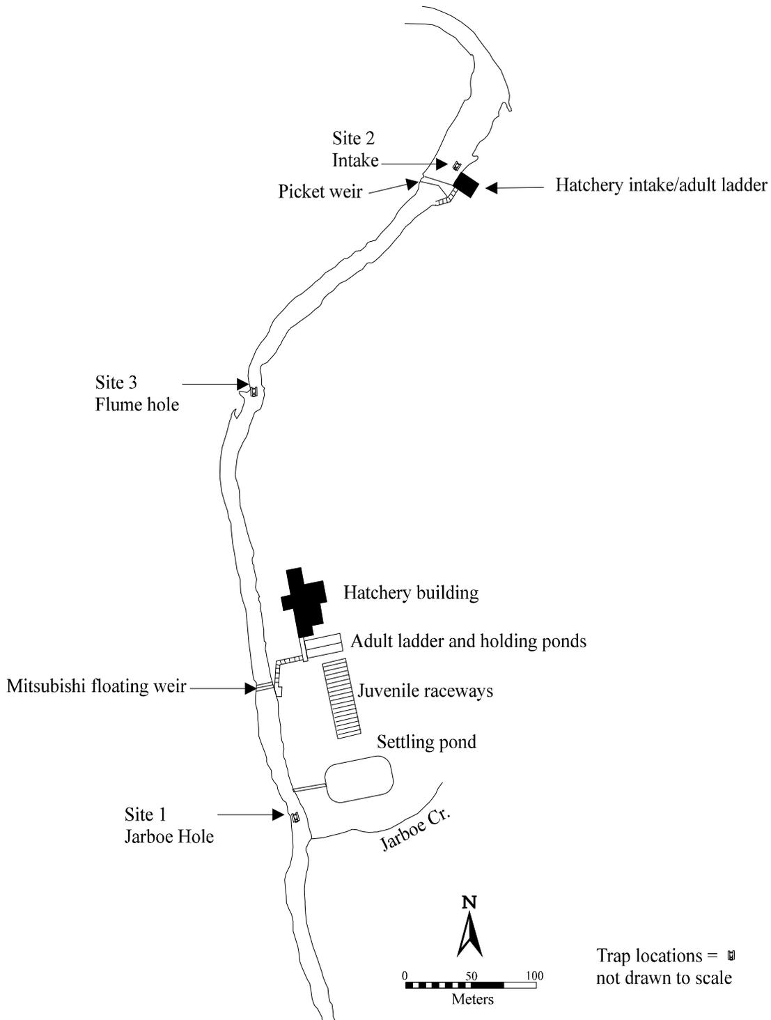
Figure 4. Locations of the rotary screw trap while trapping the 1994.
