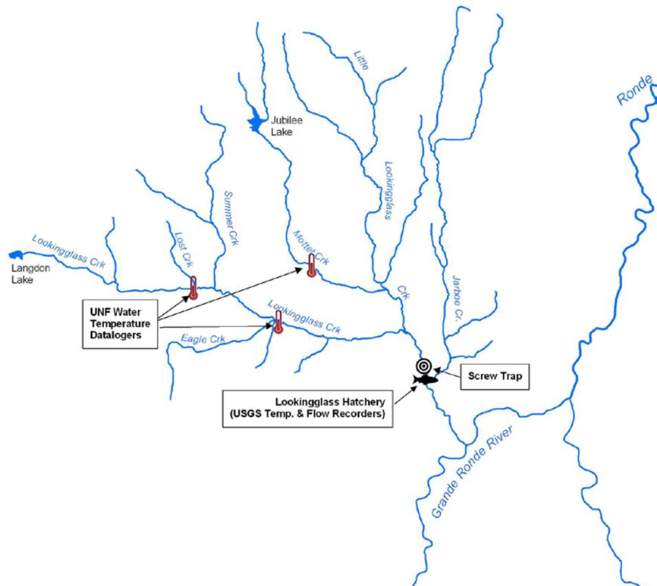
Figure 1. Map of the Lookingglass Creek basin showing the locations of major tributaries, temperature and flow recorders, screw trap and the Lookingglass Hatchery complex.
