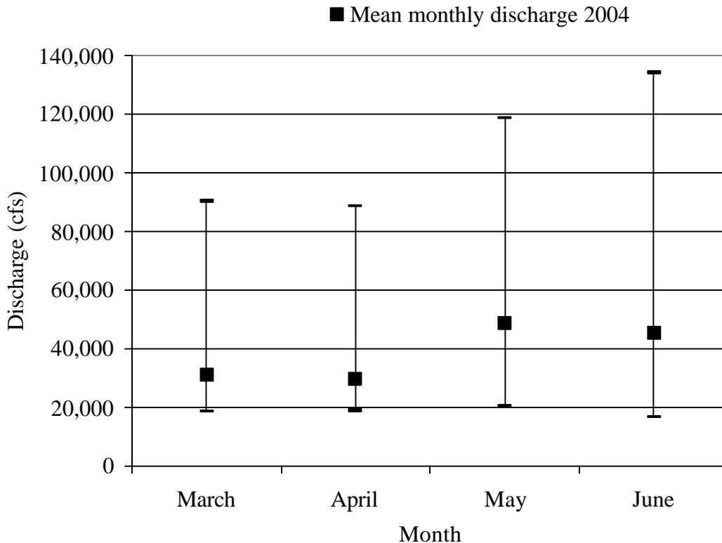
Figure 7. The average monthly discharge for the months of March, April, May, and June for 2004 at the Snake River USGS gauge 13334300. Bars indicate the minimum and maximum average monthly discharge values observed from 1959 to 2004. USGS discharge data is provisional.
