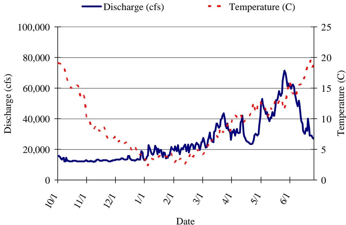
Figure 6. The average daily discharge and temperature at the Snake River gauge 13334300 from October 1, 2003 to June 30, 2004. USGS discharge data is provisional.
