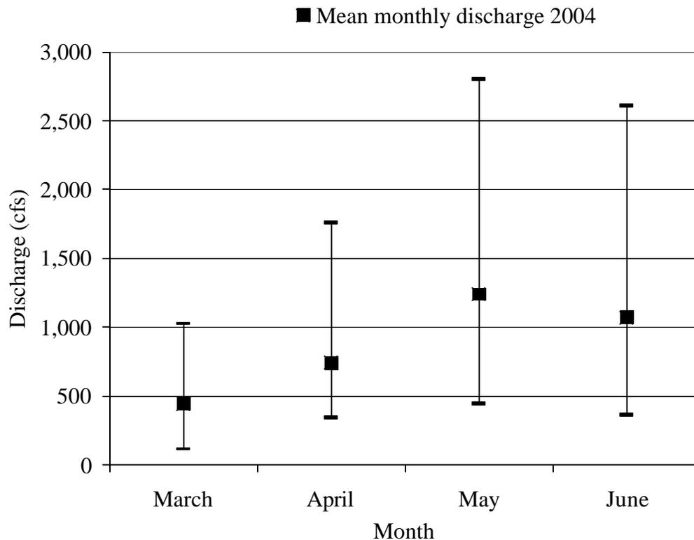
Figure 5. The average monthly discharge for the months of March, April, May, and June for 2004, at the Imnaha River USGS gauge 13292000. Bars indicate the minimum and maximum average monthly discharge values observed from 1929 to 2004. USGS discharge data is provisional.
