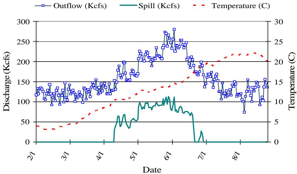
Figure 11. Measurements of outflow, spill, and mean temperature at McNary Dam from February 1 to August 29, 2004. Data was obtained online at <http://www.cbr.washington.edu/dart/>.
