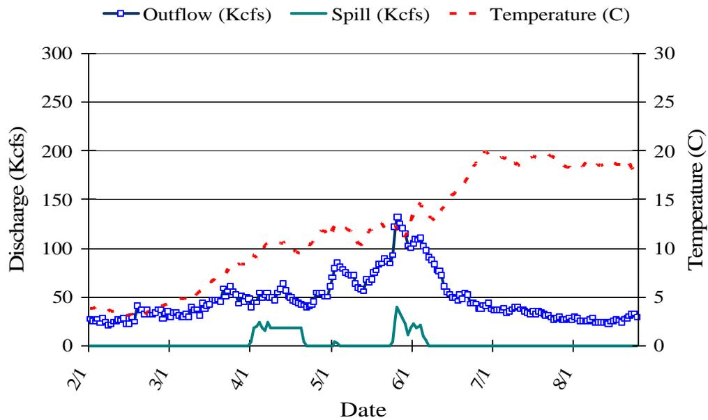
Figure 8. Measurements of outflow, spill, and mean temperature at Lower Granite Dam from February 1 to August 29, 2004. Data was obtained online at <http://www.cbr.washington.edu/dart/>.
