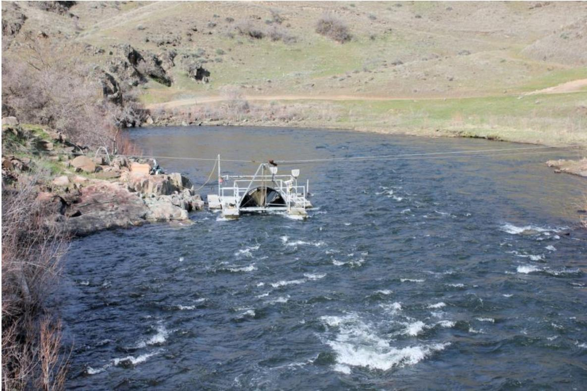
Figure 3. The Imnaha River trap (2.1m diameter) in operation.
