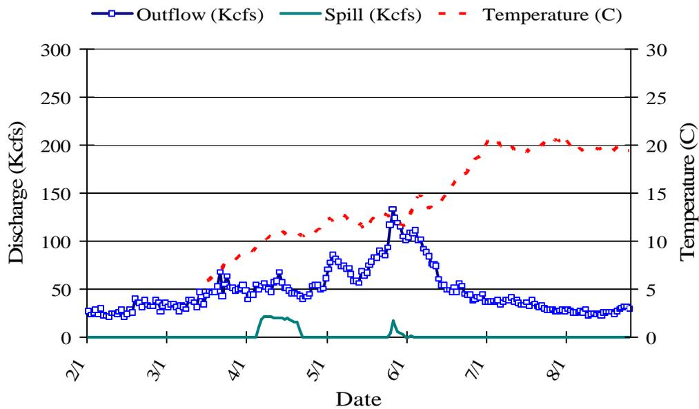
Figure 9. Measurements of outflow, spill, and mean temperature at Little Goose Dam from February 1 to August 29, 2004. Data was obtained online at <http://www.cbr.washington.edu/dart/>.
