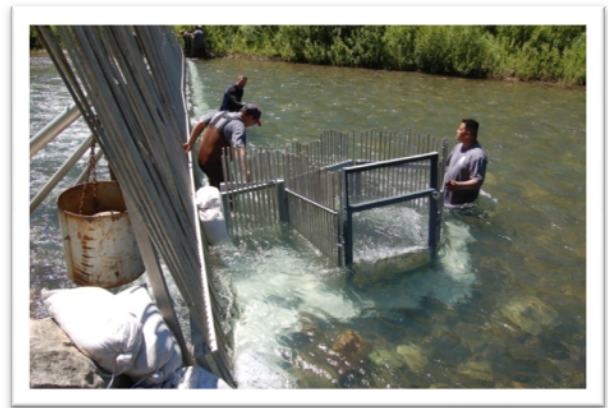
Figure 3. Initial trap box used on Pole Flat Weir.
