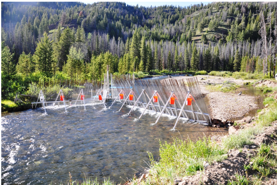
Figure 16. Photo of Five Mile weir, fish trap, live-wells, and workstation.
