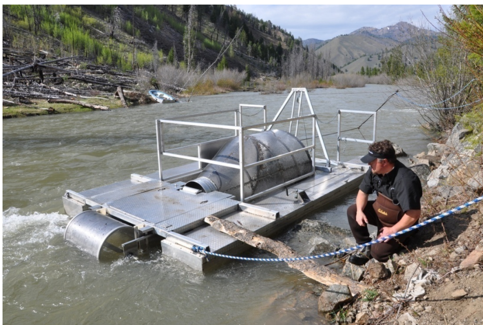
Figure 2. Yankee Fork rotary screw trap, May 17, 2012.
