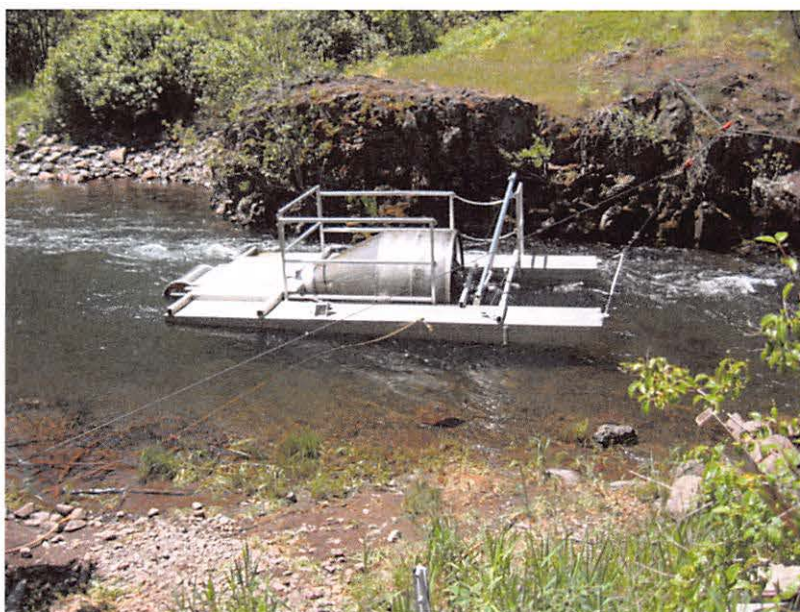
Figure 4. Lookingglass Creek rotary screw trap (1.5 m diameter) at rkm 4.0, just below the Lookingglass Hatchery adult weir and trap.
