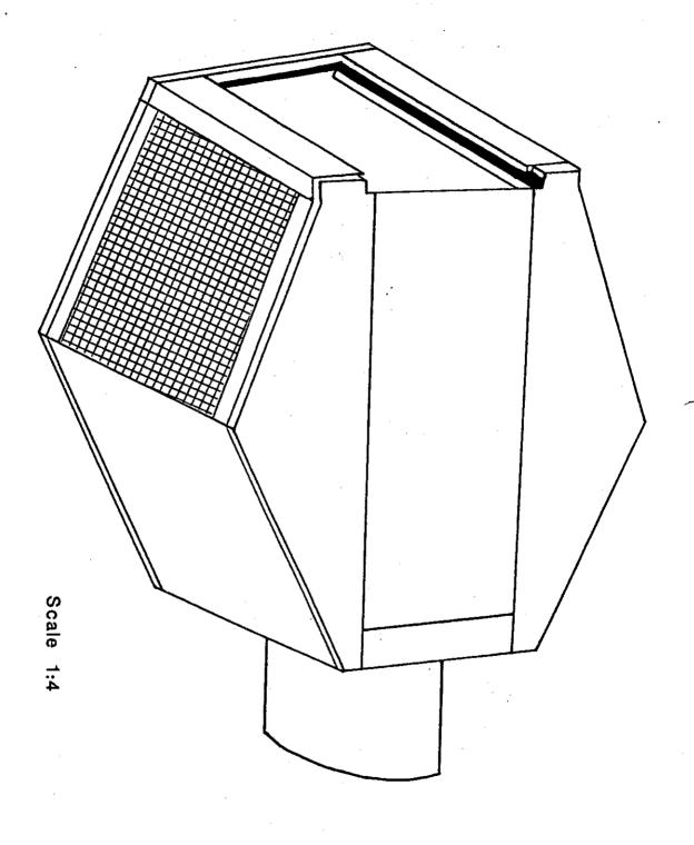
Figure 1. Trap box used to capture fry from redds capped in Catherine Creek, Oregon.
