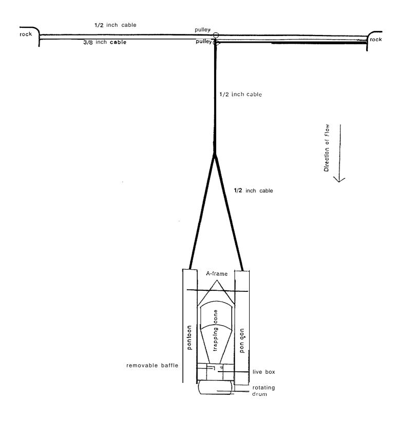
Figure 2. Diagram of screw trap.
