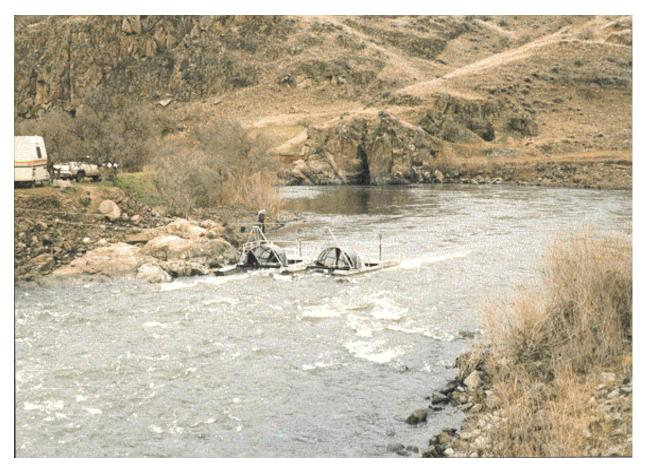
Figure 2. The lower Imnaha trap site with two rotary screw traps operating. The traps are in position 3. Trap A is on the left and trap B is on the right.
