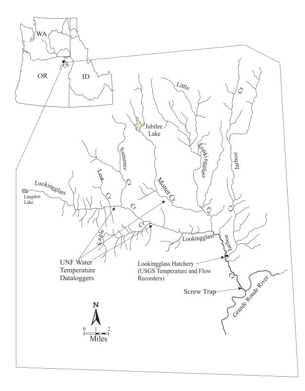
Figure 1. Map of the Lookingglass Creek basin showing the locations of major tributaries, temperature and flow recorders, screw trap and the Lookingglass Hatchery complex.
