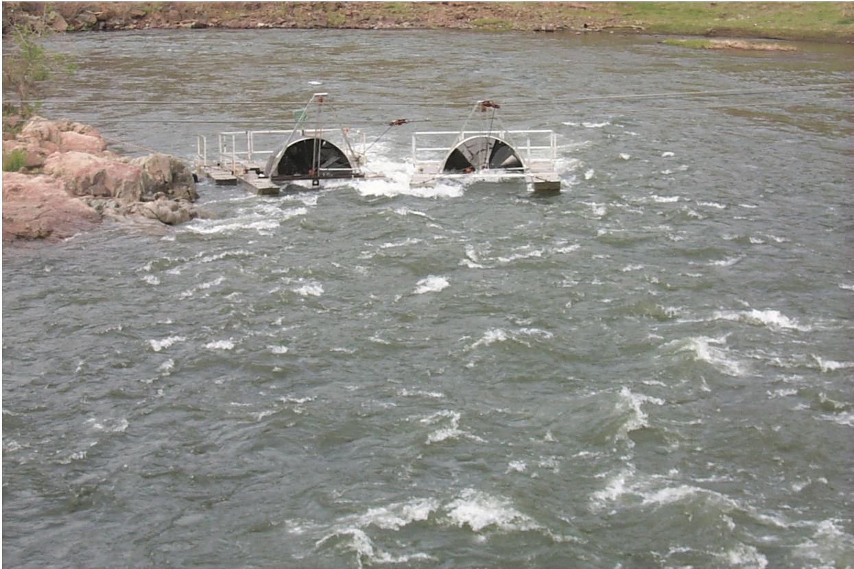
Figure 3. The lower Imnaha River trap site with two rotary screw traps operating. Trap A is on the left and trap B is on the right.
