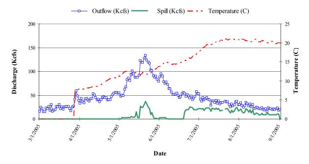
Figure 10. Measurements of outflow, spill, and mean temperature at Lower Monumental Dam from March 1 to September 1, 2005. Note that temperature did not begin recording until March 28. Data obtained online at <a href="http://www.cbr.washington.edu/dart/">http://www.cbr.washington.edu/dart/</a>.
