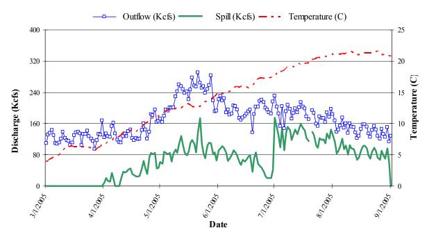
Figure 11. Measurements of outflow, spill, and mean temperature at McNary Dam from March 1 to September 1, 2005. Data obtained online at <a href="http://www.cbr.washington.edu/dart/">http://www.cbr.washington.edu/dart/</a>.
