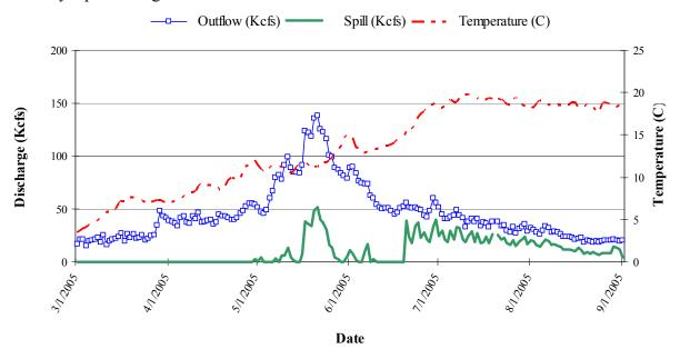
Figure 8. Measurements of outflow, spill, and mean temperature at Lower Granite Dam from March 1 to September 1, 2005. Data obtained online at <a href="http://www.cbr.washington.edu/dart/">http://www.cbr.washington.edu/dart/</a>.
