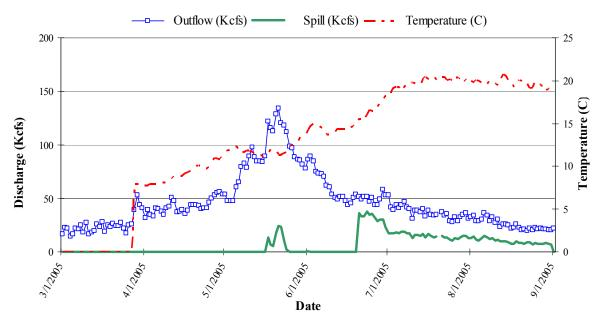
Figure 9. Measurements of outflow, spill, and mean temperature at Little Goose Dam from March 1 to September 1, 2005. Note that temperature did not begin recording until March 28. Data obtained online at <a href="http://www.cbr.washington.edu/dart/">http://www.cbr.washington.edu/dart/</a>.
