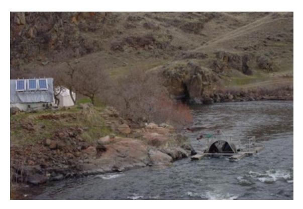
Figure 3. The Imnaha River juvenile emigrant trap site with a rotary screw trap operating.
