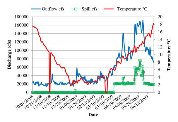
Appendix O. Measurements of outflow, spill, and mean temperature at Lower Granite Dam from October 1, 2008 to July 1, 2009. Data obtained online at <a href="http://www.cbr.washington.edu/dart/">http://www.cbr.washington.edu/dart/</a>. cfs – cubic feet per second, °C – degrees Celsius.
