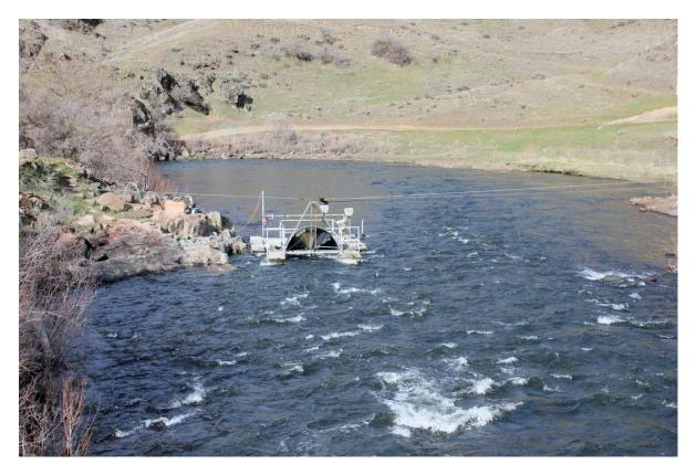
Figure 1.3. The Imnaha River juvenile emigrant trap rotary screw trap in operation.
