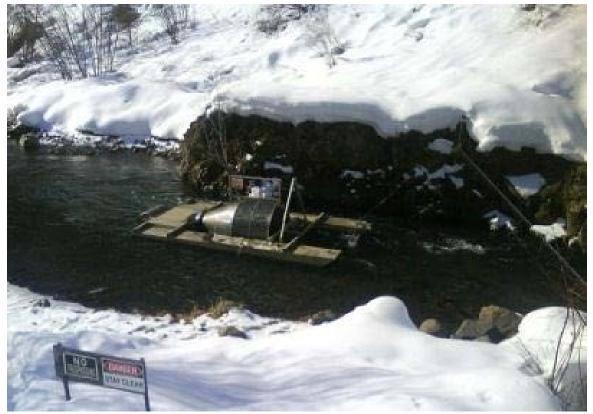
Figure 8. Rotary screw trap located at rkm 4.0 on Lookingglass Creek.
