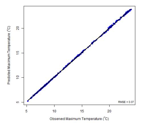
Appendix E6. Predicted maximum water temperature values vs. observed maximum water temperature values used for infilling at the Klamath River Blakes Riffle (KRTG) focal site, with observed data at USGS gage 11530500, with root mean square error (RMSE) as a measure of the difference between the predicted and reference values.
