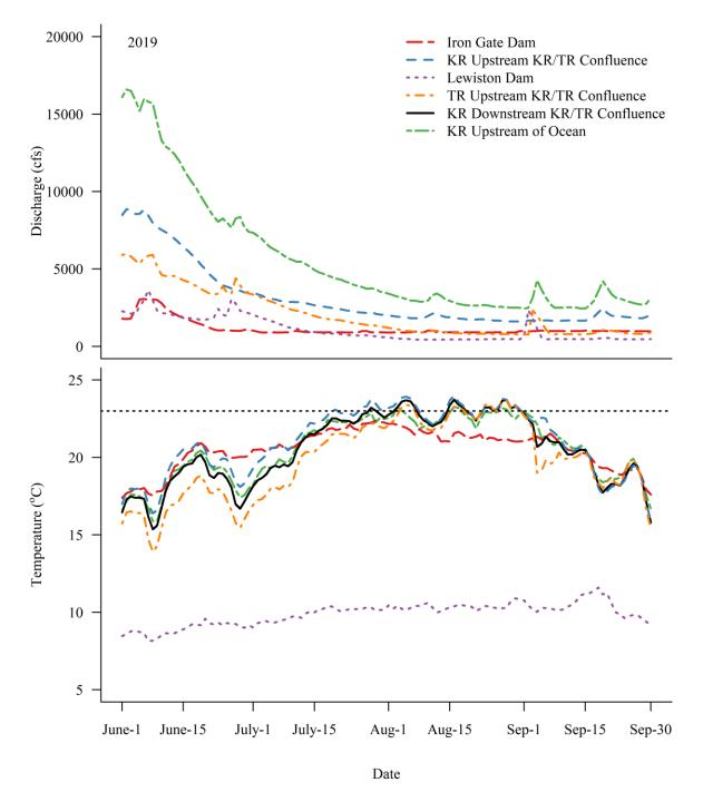
Figure 3. River discharge (cfs) at five locations and daily mean water temperature (°C) at six locations in the Klamath River (KR) and Trinity River (TR) before, during, and after supplemental releases from Trinity Reservoir and Iron Gate Dam, June 1 – September 30, 2019. Horizontal dotted black line on the bottom graph represents 23°C criteria. U.S. Fish and Wildlife Service water temperature monitoring sites are just downstream of U.S. Geological Survey gages recoding flows.
