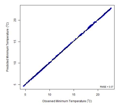
Appendix E5. Predicted minimum temperature values vs. observed minimum temperature values used for infilling at the Klamath River Blakes Riffle (KRTG) focal site, with observed data at USGS gage 11530500, with root mean square error (RMSE) as a measure of the difference between the predicted and reference values.
