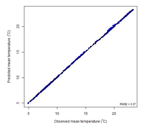
Appendix E4. Predicted mean water temperature values vs. observed mean water temperature values used for infilling at the Klamath River Blakes Riffle (KRTG) focal site, with observed data at U.S. Geological Survey gage 11530500, with root mean square error (RMSE) as a measure of the difference between the predicted and observed values.
