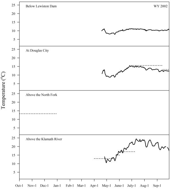
Appendix B1. Daily mean water temperatures at focal Trinity River monitoring locations, October 1, 2001–September 30, 2002. Black line = daily mean water temperatures in water year (WY) 2002; gray line = historical daily mean water temperatures; black dotted line = water temperature objectives. Sections that are blank indicates no data exists at that site for the period.
