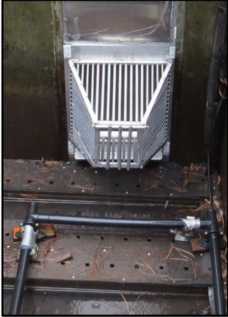
Photo 4. Photo of the new trap fyke and temporary antenna (secured to the floor of the trap) 2020.
