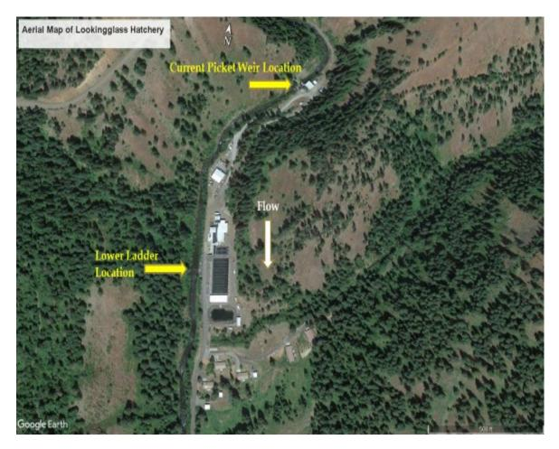
Figure 4. Aerial imagery showing the current picket weir location and the location of the lower ladder used for collections in 2021.
