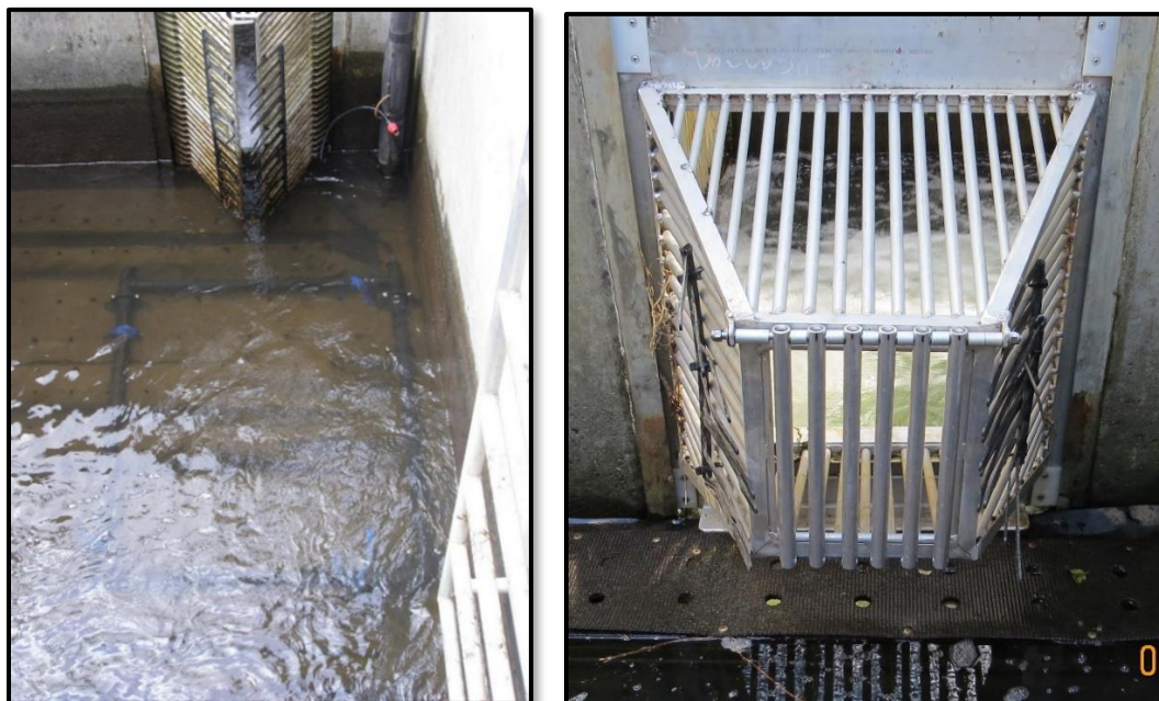
Photo 3. Photo of the temporary trap antenna operated in 2021. Note: the antenna location is the same, but the photo shows the old fyke entrance. The photo to the right shows the new fyke as installed in 2020.
