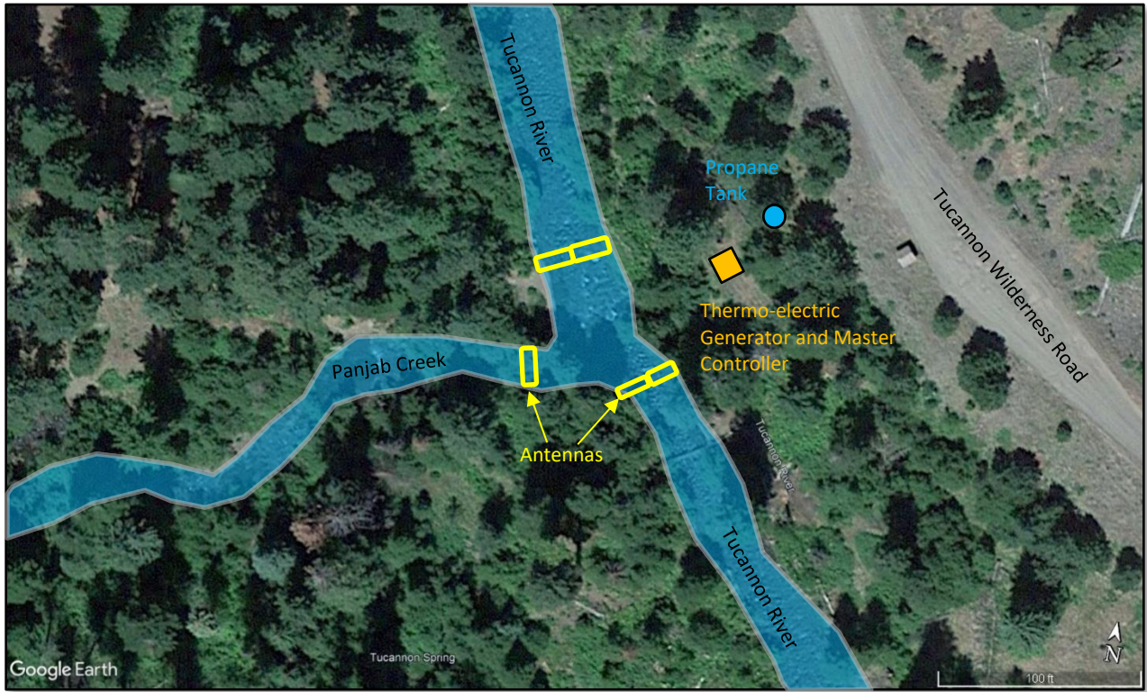
Photo 4. Configuration of the Panjab Creek PIT Tag Array Site (TPJ).
