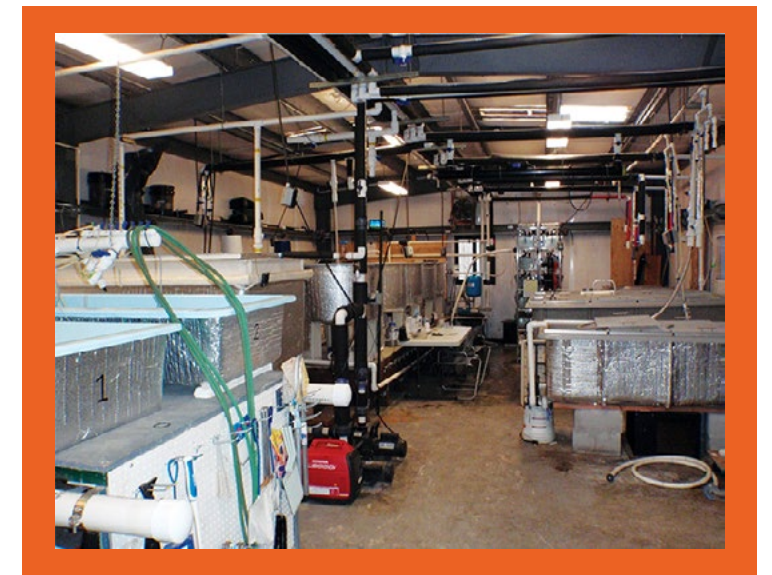
The California Nevada Fish Health Center wet laboratory has tanks and temperature controls that are used in applied research projects. Credit: USFWS
