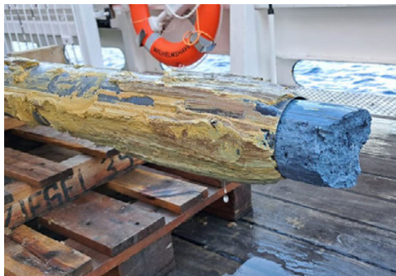
Serpentinite mud extruding from a gravity corer barrel. Photo: MARUM-Center for Marine Environmental Sciences
