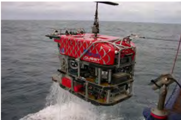
Quest 4000 ROV for deep-sea exploration. Photo: NOAA
