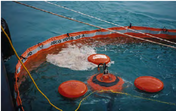
The USCG uses special skimmers to contain and recapture fuel spills. Photo: LCDR John S. Stewart /USCG
