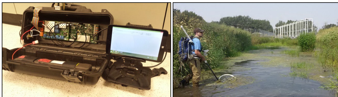
Figure 7. An IS1001ACN-based mobile PITpack reader system. (A) The PITpack reader is comprised of a waterproof Pelican case, a Windows-based tablet mounted in a harness, a detection alarm, and a lithium-ion battery. (B) Scanning a drained Feed Diversion Canal with a PITpack detection wand, 2015.
