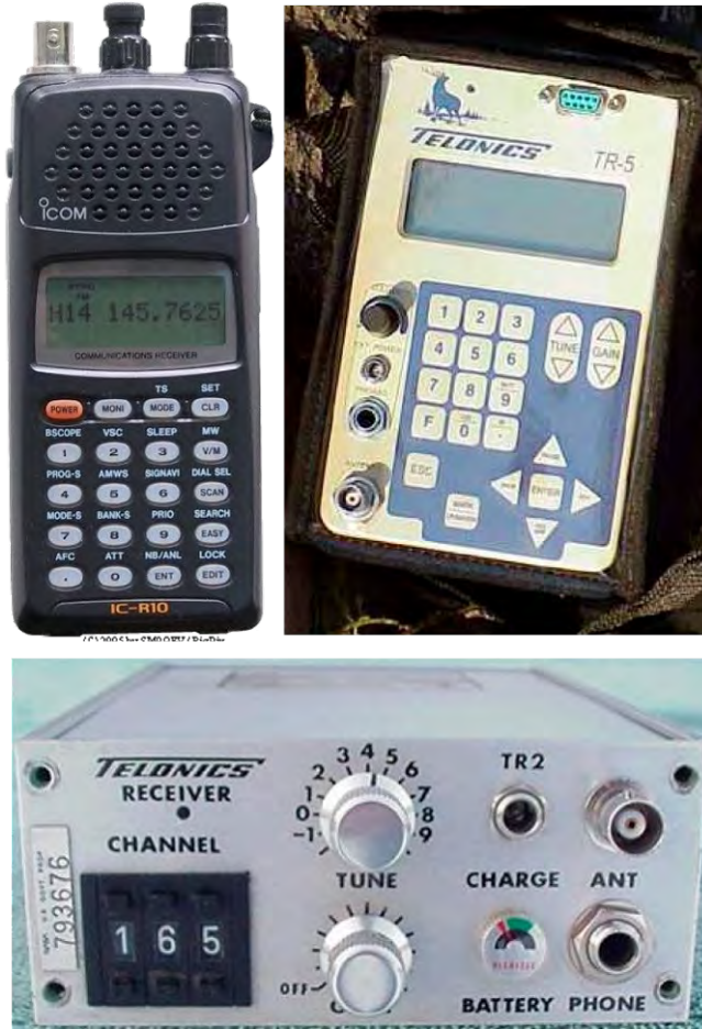
Figure 3. Examples of three typical VHF receivers used in radio telemetry. The Icom IC-R10 (top left) is a multi-band VHF receiver, while the Telonics TR-5 (top right) and Telonics TR-2 (bottom) operate in more limited frequency ranges.
