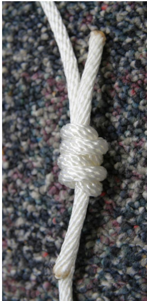
Fig. 5. Fisherman's bend. This knot is likely more secure in a nylon rope than polypropylene.
