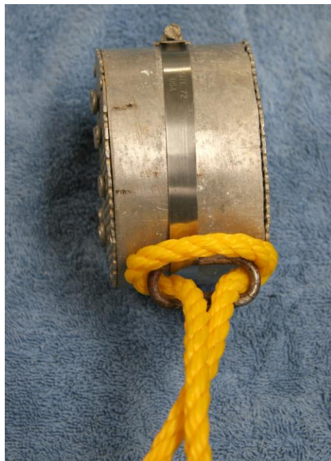
Fig. 4. Anchor line looped around PEMD shackle
