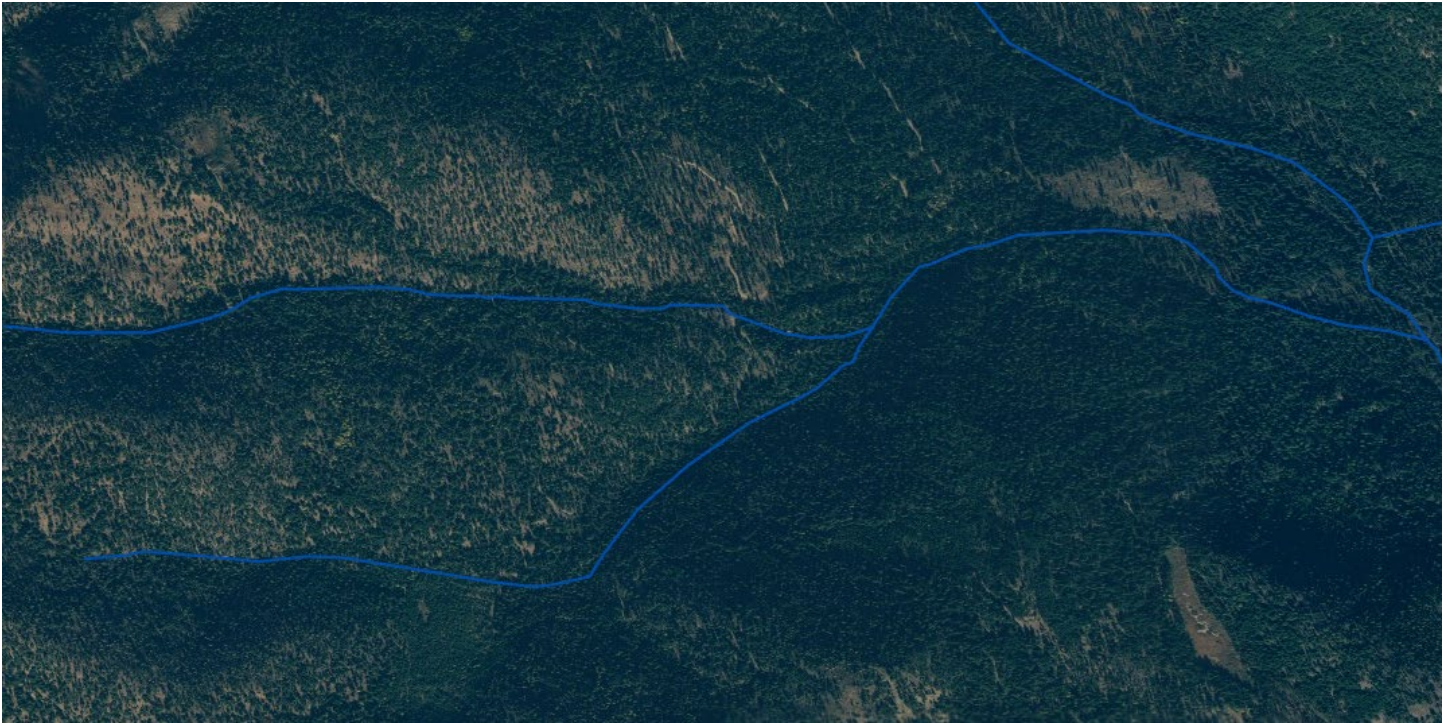
Figure 3. HRDS streams or rivers obscured by tree canopy, shadow, snow, etc. should be included in the polygonal dataset unless there is sufficient ancillary data to suggest the feature is no longer an active stream.
