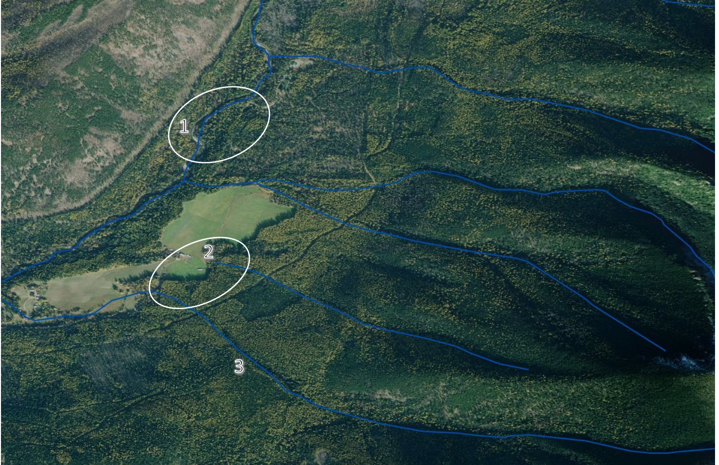
Figure 10. The HRDS features represented in this example illustrate several mapping considerations as described in the guidelines above: 1) improper alignment—if the HRDS feature is buffered as is, the resulting polygon will not meet horizontal standard requirements; 2) disconnected features—the riverine feature should connect to another wetland feature unless there is sufficient ancillary data to show there is no surface water connection; and 3) feature obscurity—features obscured by tree canopy should remain in the dataset unless there is sufficient ancillary data to support their removal.
