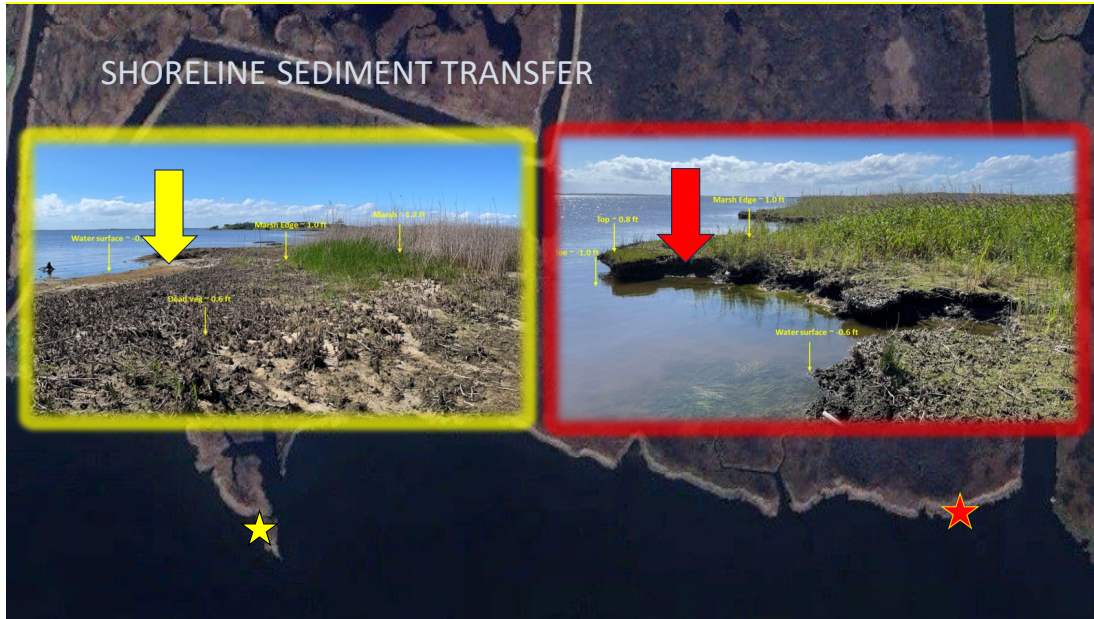
Figure 4. Shoreline Sediment Transfer. Shoreline sediment deposited 1,300 yards west of Corey's ditch (Yellow Arrow) showing a gradual shoreline. No shoreline sediment being deposited near the mouth of Corey's ditch (Red Arrow) showing a vertical shoreline.
