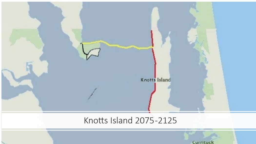
Figure 10. View of Knotts Island if the Mackay NWR marshes are gone. To ensure access to and from Knotts Island, NCDOT will likely need to raise and rock the entire length of the causeway to combat waves over topping the road (yellow line). The entire west facing shoreline of Knotts Island will need shoreline protection to eliminate erosion of the island (Red line).
