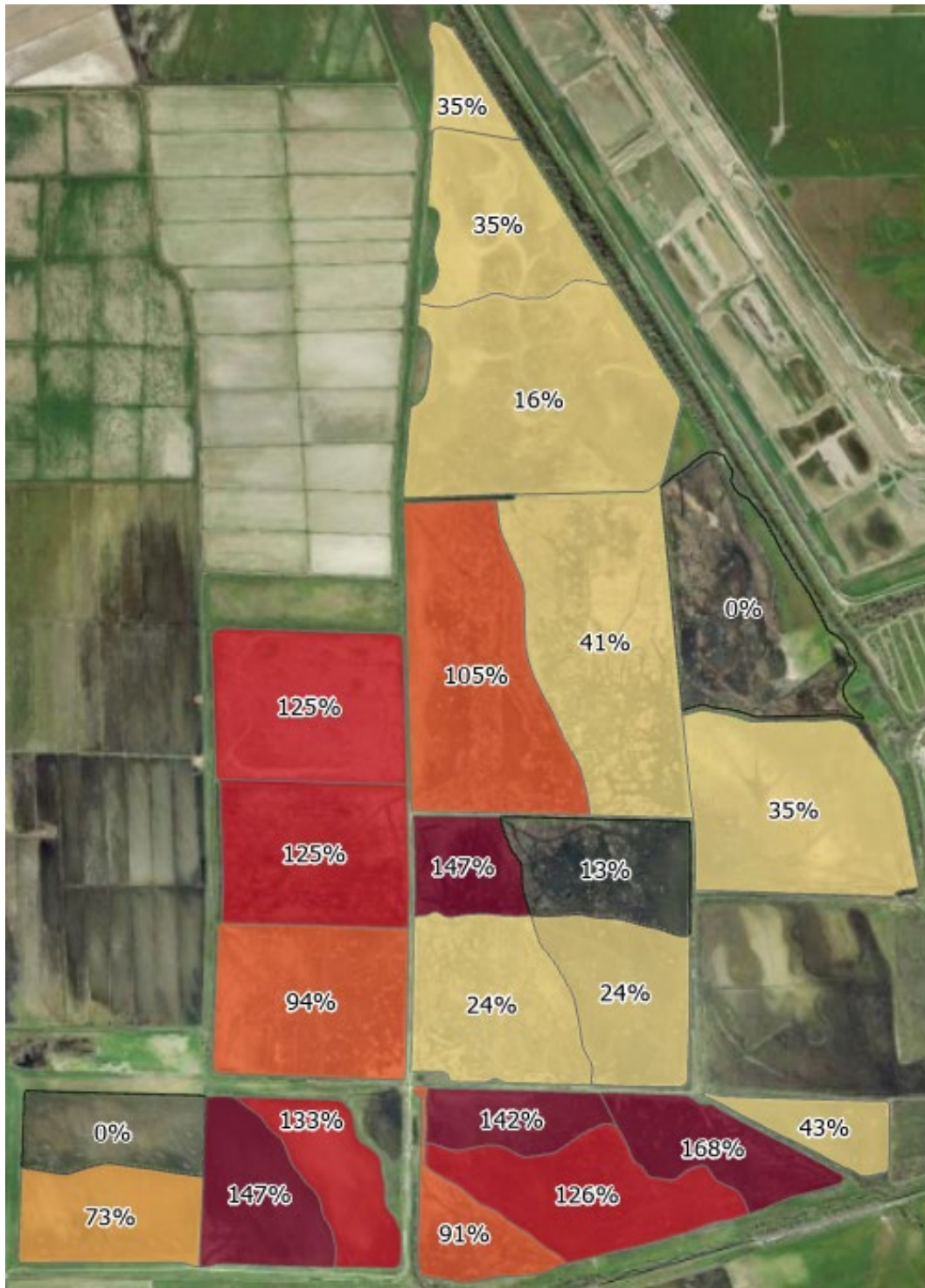
Figure 4. Proportional increase in 6+ inch flood event count over baseline conditions attributable to the Big Notch Project during maximum impact years. Maximum impact water years defined as the four years which had the largest cumulative difference in flood events between baseline and Big Notch scenarios. Values are presented by wetland unit in the North Area. Shading corresponds to values.
