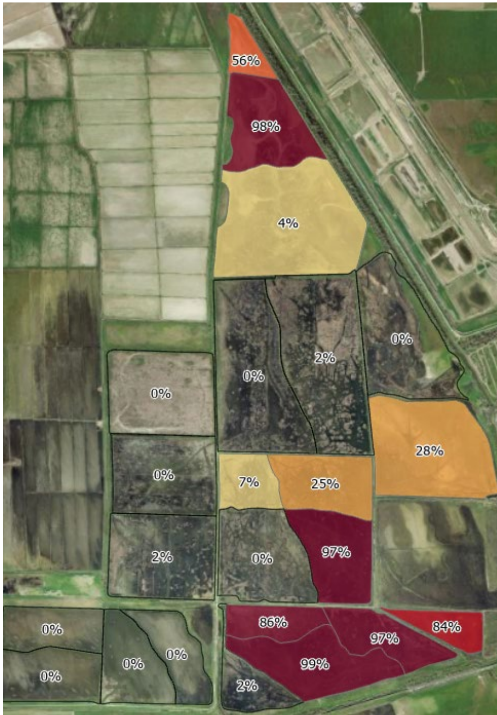
Figure 11. Proportional increase in greater-than-berm-height flood duration over baseline conditions attributable to the Big Notch during maximum impact years. Maximum impact water years defined as the four years which had the largest cumulative difference in duration between baseline and Big Notch scenarios. Values are presented by wetland unit in the North Area. Shading corresponds to values.
