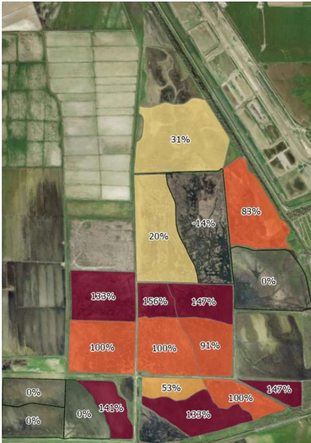
Figure 8. Proportional increase in greater-than-blind-height flood event count over baseline conditions attributable to the Big Notch Project under maximum impact years. Maximum impact water years defined as the four years which had the largest cumulative difference in flood events between baseline and big notch scenarios. Values are presented for each wetland unit in the North Area. Shading corresponds to values.
