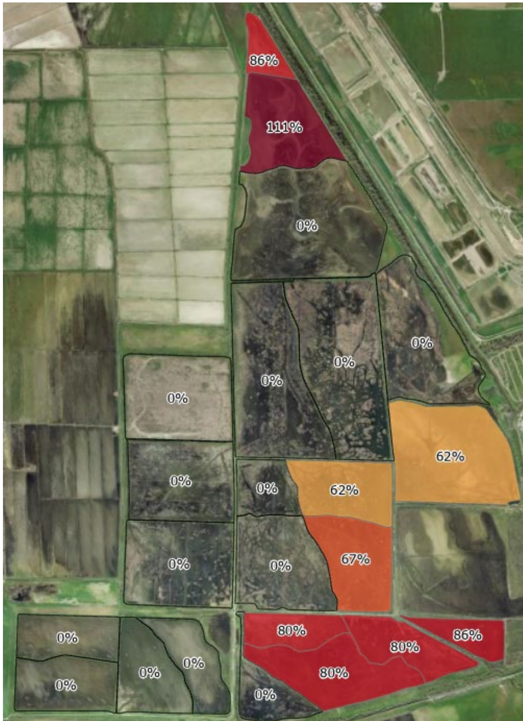
Figure 12. Proportional increase in greater-than-berm-height flood event count over baseline conditions attributable to the Big Notch during maximum impact years. Maximum impact water years defined as the four years which had the largest cumulative difference in duration between baseline and Big Notch scenarios. Values are presented by wetland unit in the North Area. Shading corresponds to values.
