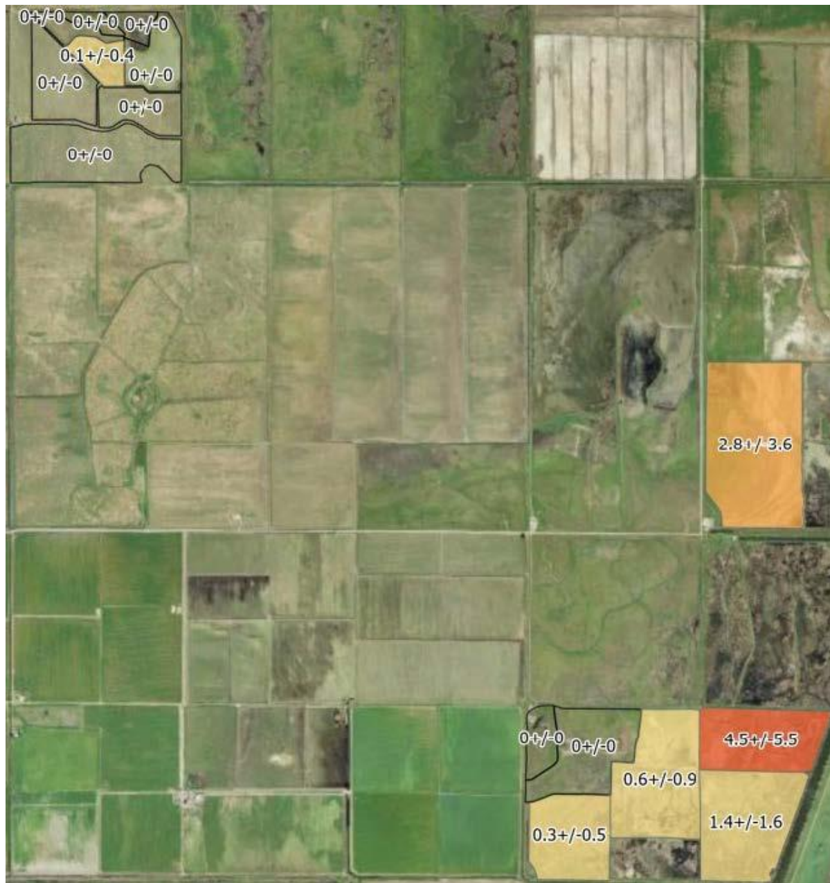
Figure 9. Averaged annual difference of greater-than-berm-height flood duration between baseline and Big Notch scenarios, for wetland units in the South Area. Unit specific days are presented, followed by standard deviation values. Shading corresponds to values.
