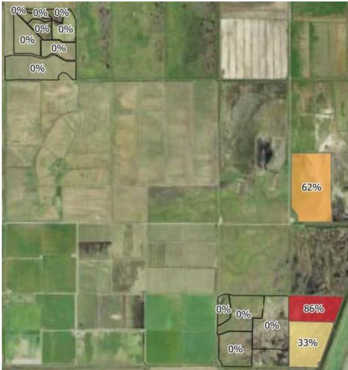
Figure 12. Proportional increase in greater-than-berm-height flood event count over baseline conditions attributable to the Big Notch during maximum impact years. Maximum impact water years defined as the four years which had the largest cumulative difference in duration between baseline and Big Notch scenarios. Values are presented by wetland unit in the South Area. Shading corresponds to values.
