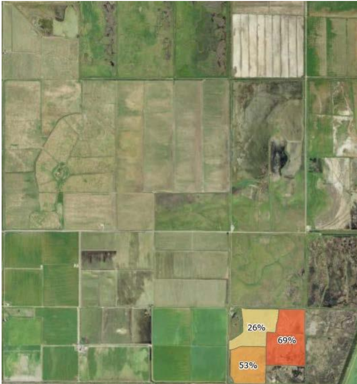
Figure 7. Proportional increase in greater-than-blind-height flood duration over baseline conditions attributable to the Big Notch under maximum impact years. Maximum impact water years defined as the four years which had the largest cumulative difference in duration between baseline and big notch scenarios. Values are presented by wetland unit in the South Area. Shading corresponds to values.
