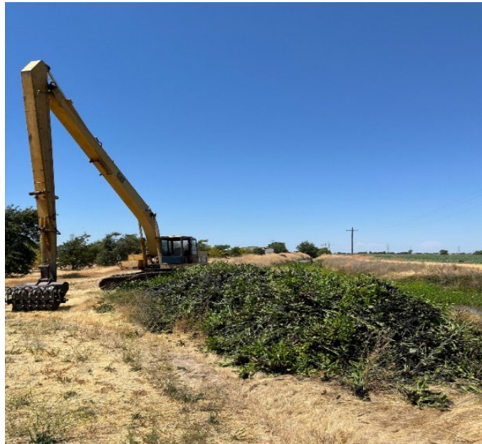
Figure 7. Biomass removal could include mechanical removal of aquatic invasive plants using heavy equipment on the bank of a water feature.
