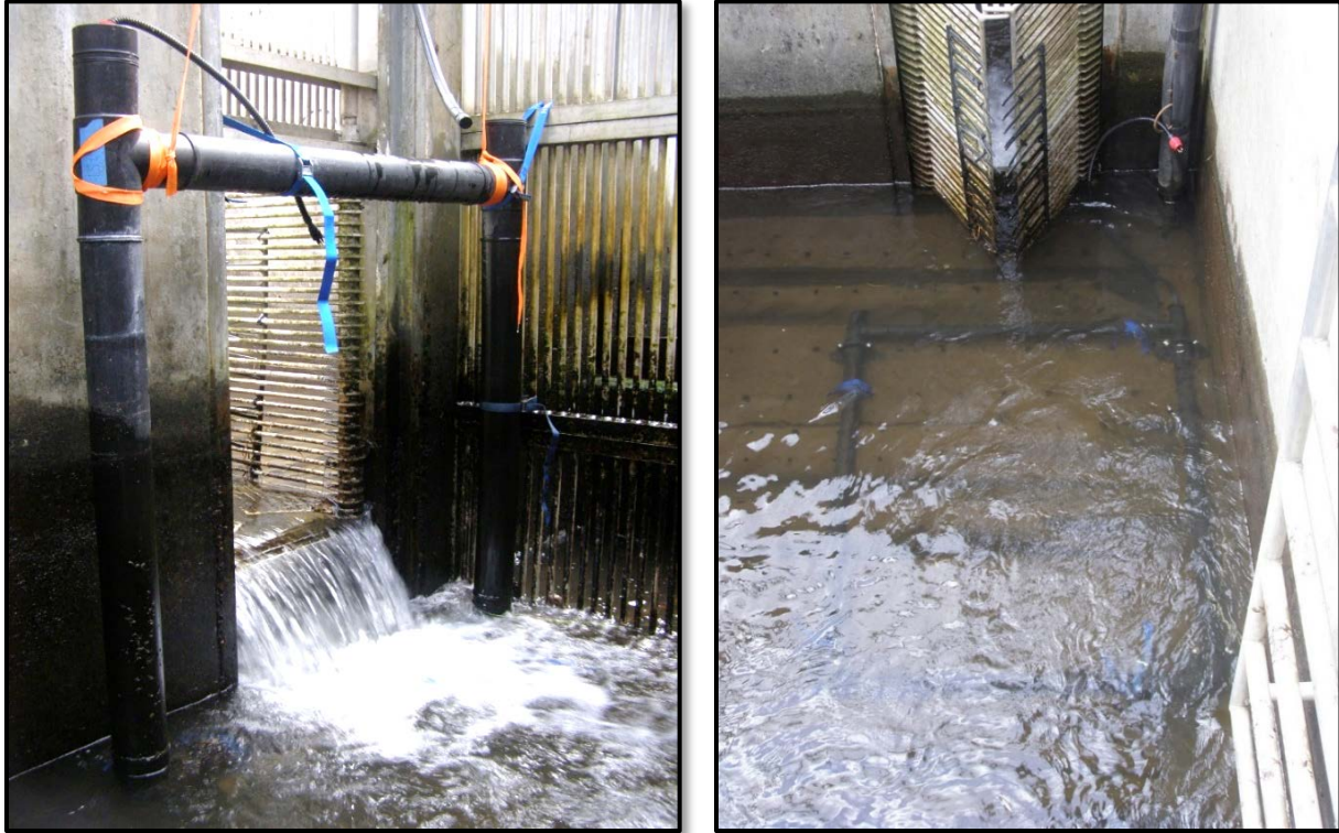
Photo 3. Photos of temporary antennas installed in 2019. (A) is the antenna placed immediately in front of the trap entrance, and (B) was mounted on the trap floor immediately in front of the trap throat. Note: the normal water level when the trap is in operation in both photos can be visually seen by the wetted walls.
