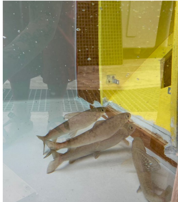
After fish are exposed to the flume holding area for 24 hours, a gate is opened and fish are allowed to navigate through the entire flume channel. Here, a group of grayling is stacking up just below the first step in the experimental flume. PIT tag antennas are located at several locations throughout the flume channel recording fish as they travel.
