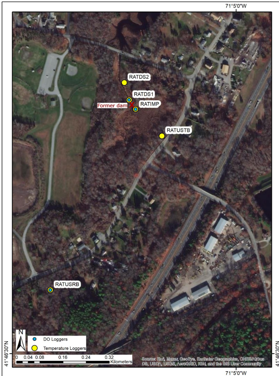
Figure A13.1. Map of temperature and dissolved oxygen logger locations in Rattlesnake Brook, Fall River, MA. Macroinvertebrates were sampled in approximately 100m sections around RATUS, RATIMP, and RATDS1 loggers. See Figure 1 in Study Design section for location within Massachusetts. Esri World Imagery Basemap accessed 10/18/2022.
