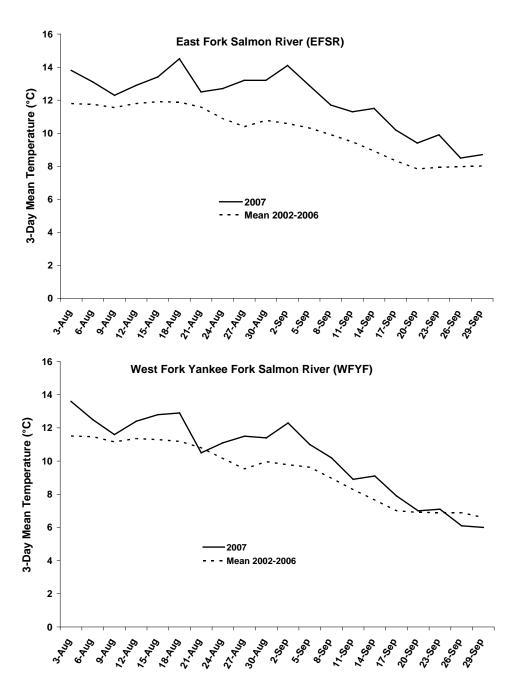
Figure 6. Three-day moving average temperatures for the East Fork Salmon River (EFSR) and the West Fork Yankee Fork (WFYF) during 2007 compared to the mean for 2002-2006.
