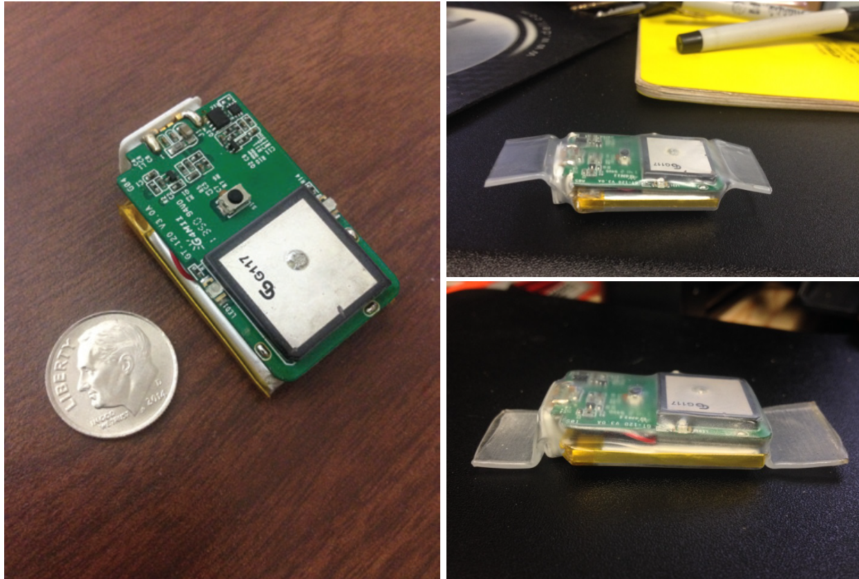
Figure 14. Photographs of i-gotU GPS tags used in this study. Left: i-GotU GT-120 GPS tag removed from original packaging. This tag type was used to track Red-tailed Tropicbirds, Wedge-tailed Shearwaters, Brown Boobies, and Red-footed Boobies in MHI, 2013–2016. Upper right: Tag sealed in heat shrink with heat shrink tabs aligned with top of tag for underside tail attachments. Lower right: Tag sealed in heat shrink with heat shrink tabs aligned with bottom of tag for attachments on top of tail or back. Note that for tail attachments beginning in 2015, one heat shrink tab was folded up against the tag to allow closer placement of the tag to the bird's body.
