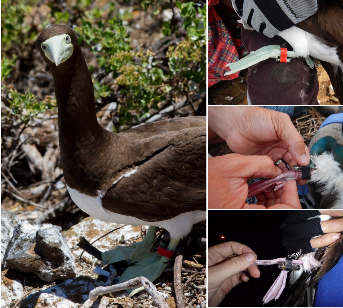
Figure 17. Example attachments of CEFAS G5 Temperature-Depth Recorders (TDRs) on seabirds in MHI, 2014–2015. TDRs were taped to the metal leg band with the pressure transducer and saltwater switch oriented towards the bird's body to avoid potential sensor damage from the bird walking on the ground. Left and top right: Brown Booby. Middle right: Red-footed Booby. Lower right: Wedge-tailed Shearwater.
