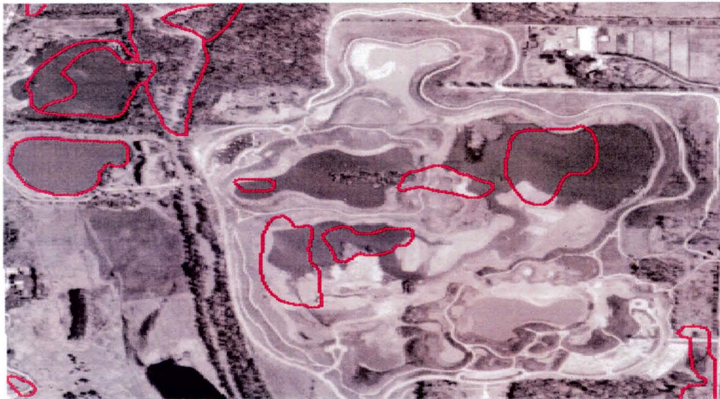
Figure 4. This aerial photograph shows a new housing development in the early stages of construction. Former wetland extent is shown by the red polygons. New water bodies are evident throughout the project area. Lands in transition, such as this example, often exhibit dramatic wetland change (Original imagery was black and white, digital orthophoto quarterquad courtesy of the State of Illinois).
