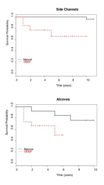
Figure 7. Kaplan-Meier survival curves for natural and TRRP-constructed side channels (upper panel) and alcoves (lower panel) in the restoration reach of the Trinity River, California. Time (years) indicates the amount of time since construction.
