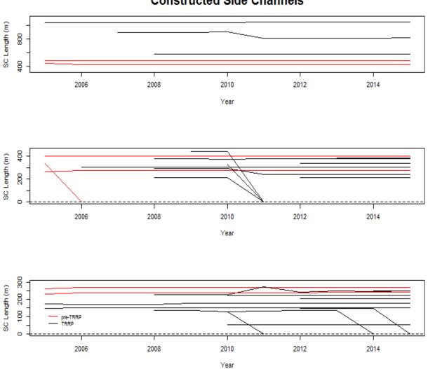
Figure B-2. Length of constructed side channels over the study period, 2005-2015. Side channel length is depicted by a line for the years the side channel is either visibly connected (>0) to or temporarily disconnected (= 0) from the mainstem Trinity River over the study period as determined by visual inspection of aerial photographs. Note, to aid visualization, constructed side channels are displayed in three panels and the y-axes are not scaled the same.
