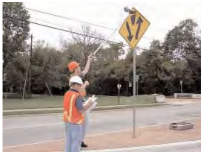
Retroreflectometers are used to measure sign retroreflectivity.
