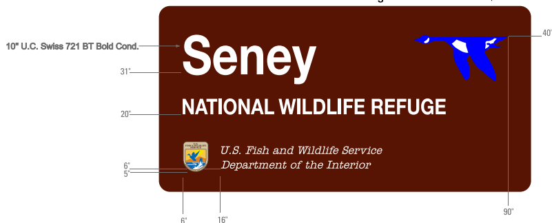
1-Line Short Name 4 x 8 Entrance Sign Measurements (from the bottom and left)
