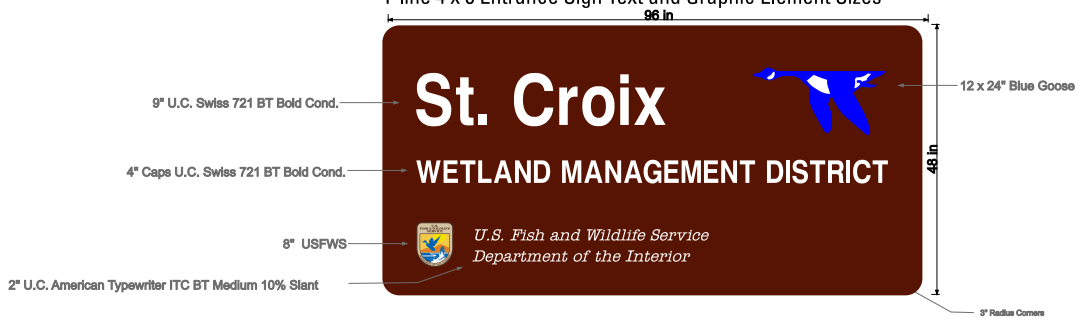
1-Line 4 x 8 Entrance Sign Measurements (from the bottom and left)
